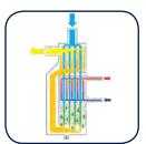
The ALU-DRY aluminum heat exchanger module has a vertical flow layout, ensuring the wet compressed air flows down and moisture is pulled by gravity to the
